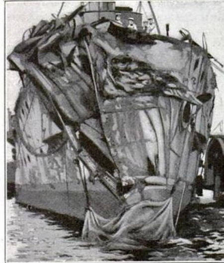
The Bow of the "Hawke," the Damage being so Great That the Ram Has Been Mashed Flat
